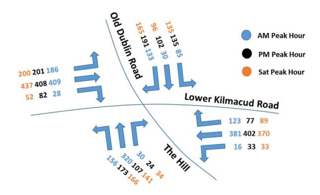
Figure 3.4 Existing Peak Hour Classified Turning Counts (vehicles)
