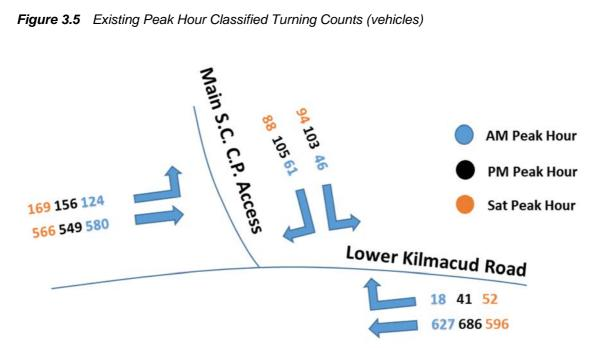
Figure 3.6 Existing Peak Hour Classified Turning Counts (vehicles)
