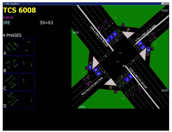
Figure 4.5 Existing Traffic Signal Plan
