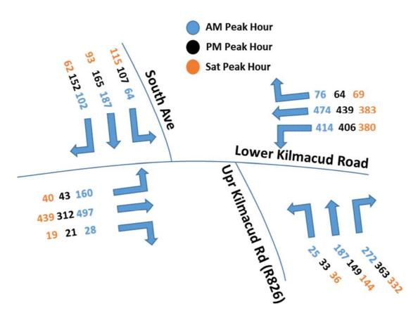
Figure 3.5 Existing Peak Hour Classified Turning Counts (vehicles)
