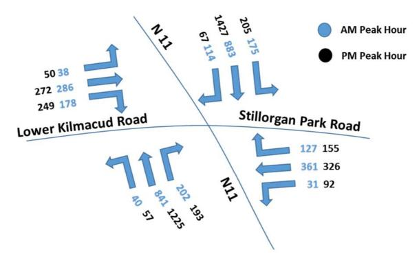
Figure 3.7 Existing Peak Hour Classified Turning Counts (vehicles)
