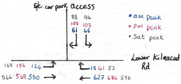
Figure 3.2 Existing Peak Hour Classified Turning Counts (vehicles)
