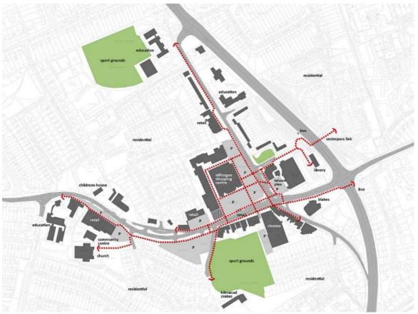
Figure 4.3: Existing Pedestrian Desire lines and Road Network
