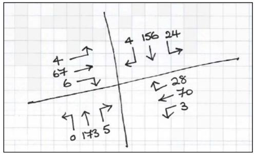
Figure 4.3 Existing 12-hour Bicycle Turning Counts
