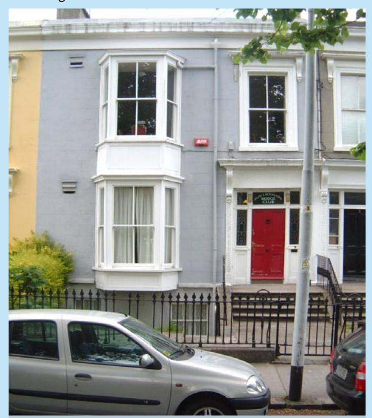
**ABOVE:** An example of the terraced two bay, two-storey over basement house on the north side, constructed with a shared chimneybreast party wall and having a paired front door with the neighbouring house.
