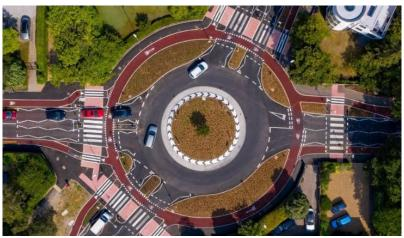
Figure 4-3 Indicative Dutch Style Roundabout Junction layout
