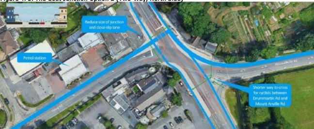
Option 3 would also include similar infrastructure changes to option 1, although would move the 2-way cycle intervention to the south side of the junction, reducing the potential for significant retaining structures on the northern side of Mount Anville Road and Taney Road. The existing left turn lanes on Taney Road and Mount Anville Road would be removed to accommodate the cycleway with left turn movements facilitated within signalised left turn lanes.
