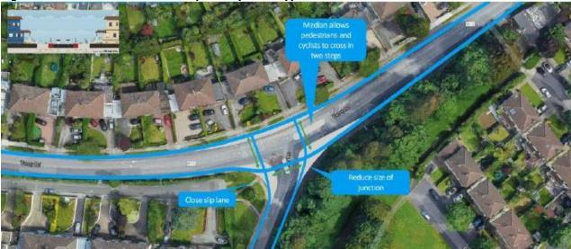
Option 2 would require those cycling along Birches Lane towards this scheme to cross with caution at the junction to pass to the north-side of the street and enter the two-way cycle track.
