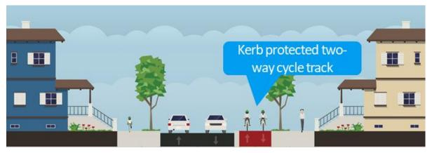
Figure 6-1 Typical one-way and two-way cross section between junctions (images: Streetmix)
