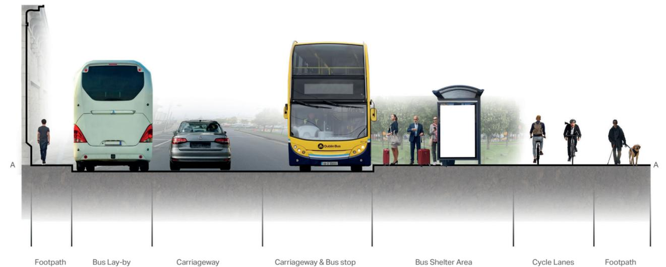
Image 1.1- Section showing cut through revised road layout along Harbour Road.
