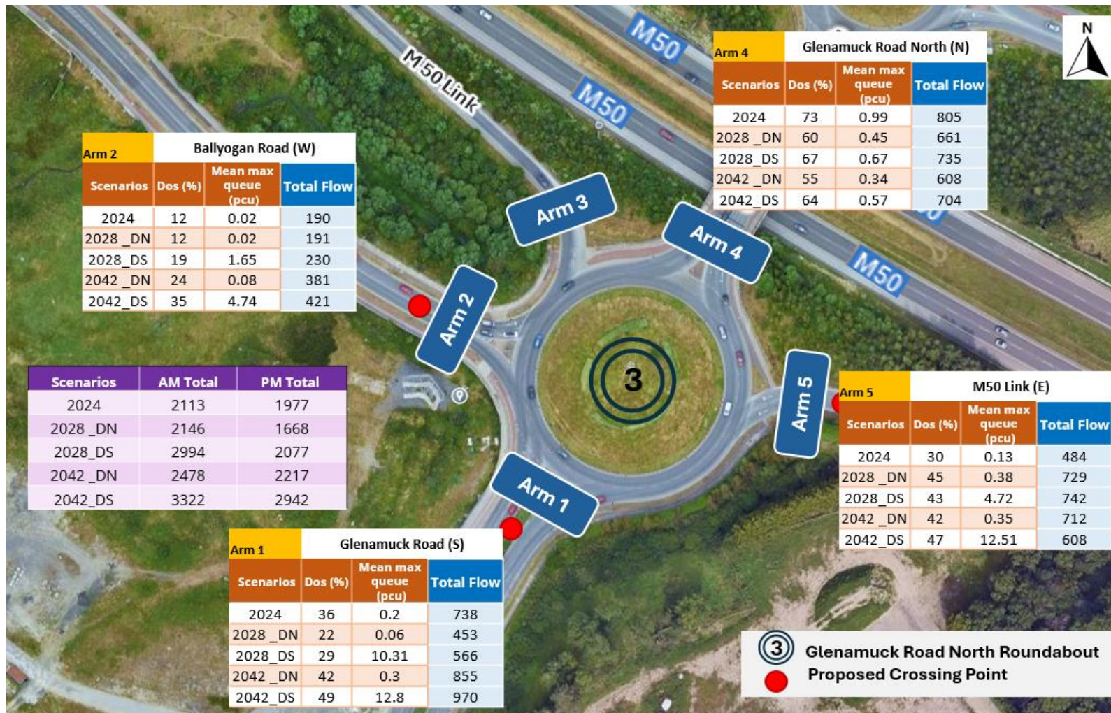
Figure 1 TRANSYT Modelling AM Results on Glenamuck North Roundabout
