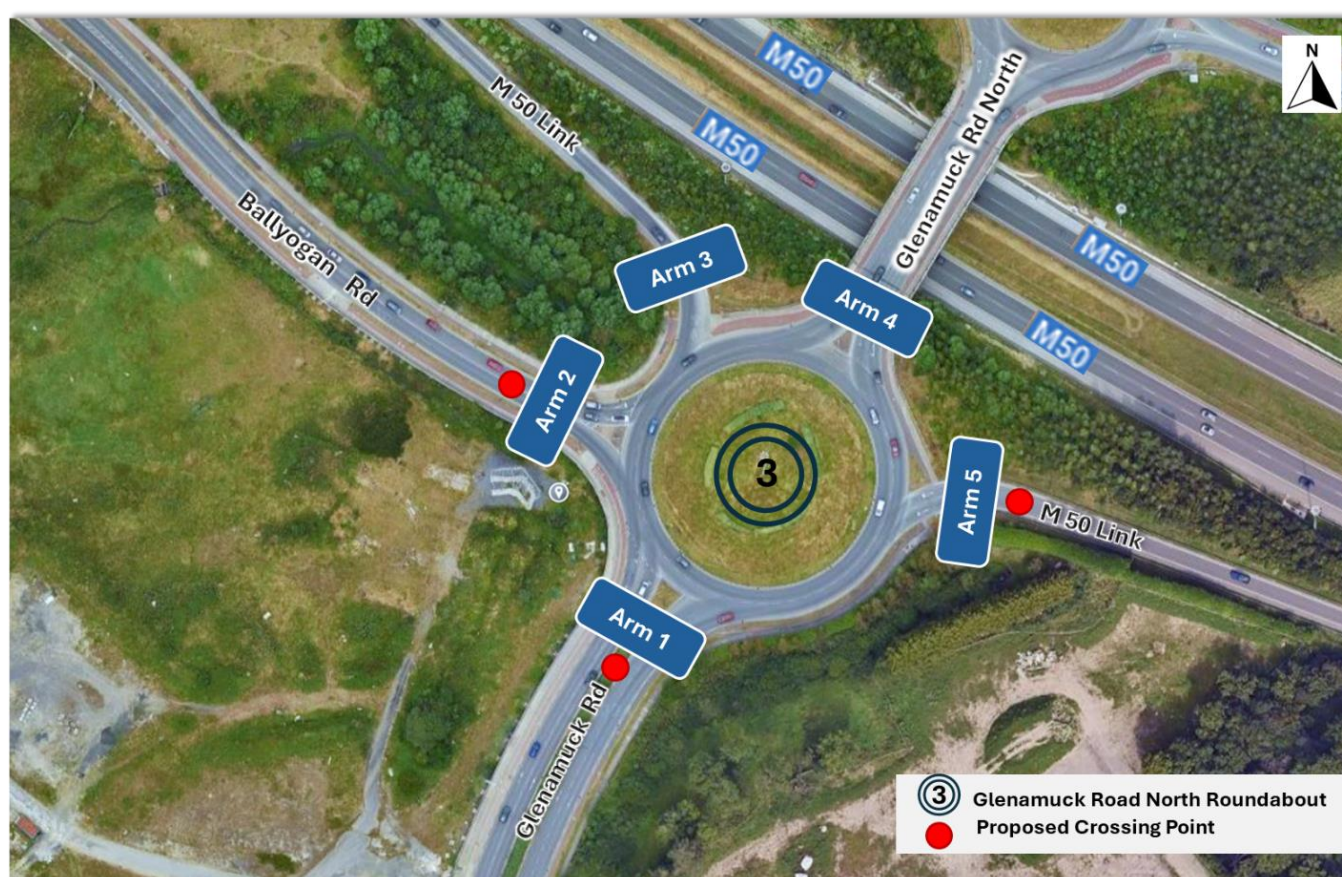
Figure 4 Existing and Proposed Layout of the Glenamuck Road North Roundabout
