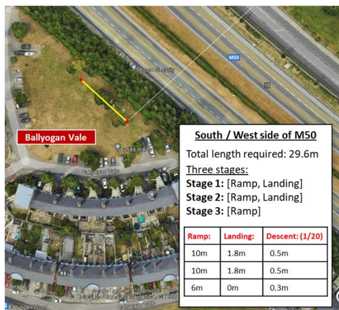
Figure 9-14 Break- down of the technical assessment of the landing area required south of the M50 for Option 3.
