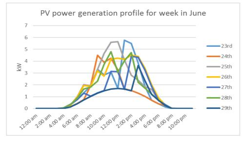
Figure 8: Profile of PV generation for sample 7 days
