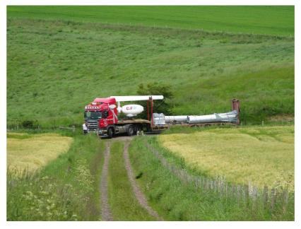
Photograph 5: Wind turbine installation. Access roads to site will need to be assessed for suitability for long vehicles.
