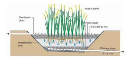
Figure 12 Schematic Cross Section of Constructed Wetland
