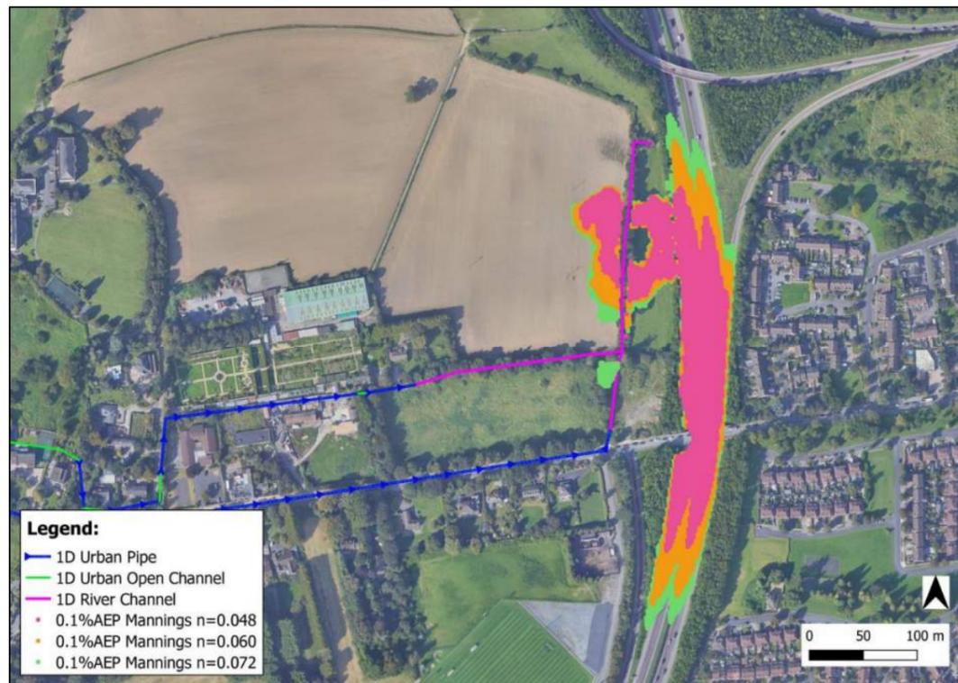
Figure 6-18: 0.1%AEP Flood Extents - Variation in Mannings n Roughness in 1D River Model
