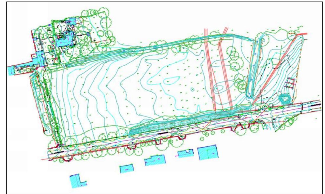
Figure 4-1: Topographic Survey Extents
