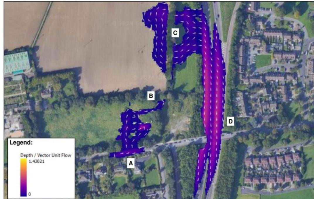
Figure 6-14: 0.1%AEP MRFS - Overland Flow Path Directions
