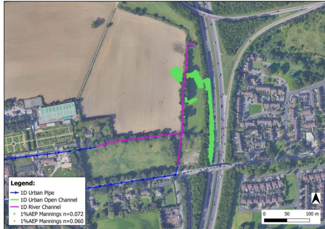
Figure 6-17: 1%AEP Flood Extents - Variation in Mannings n Roughness in 1D River Model
