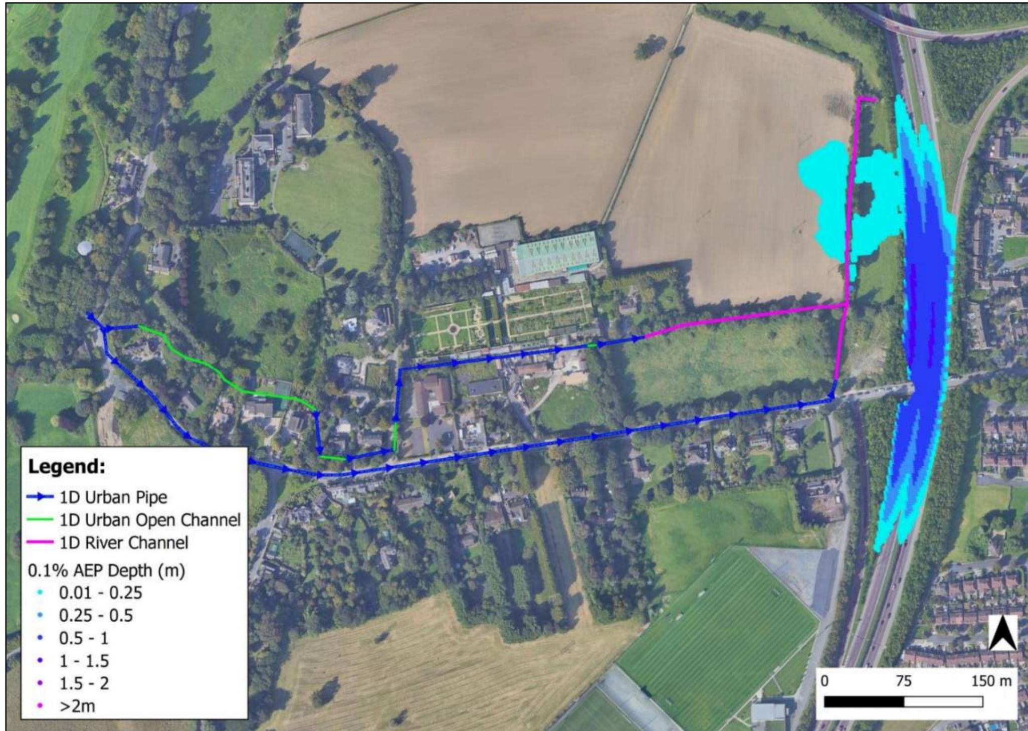
Figure 6-8: Current Scenario 0.1%AEP Flood Depth
