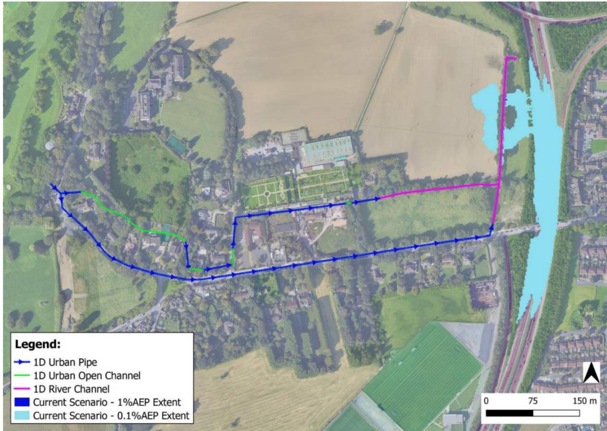
Figure 6-7: Current Scenario 1%AEP and 0.1%AEP Flood Extents
