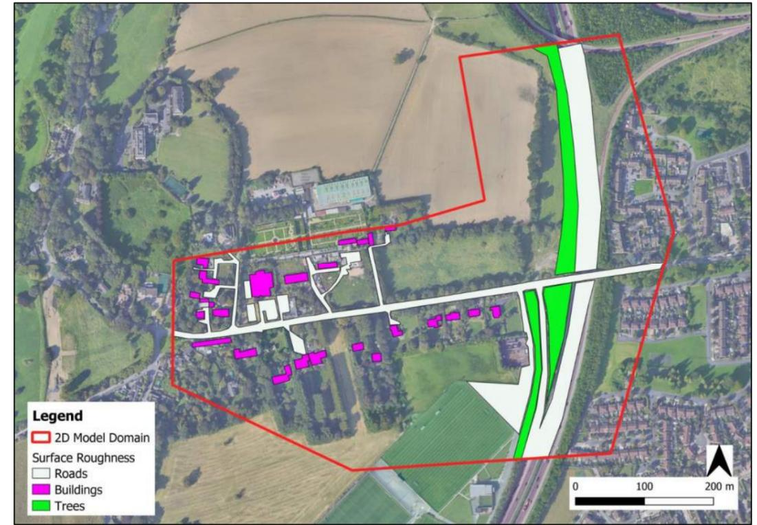
Figure 6-5: Tuflow 2D Domain Surface Roughness
