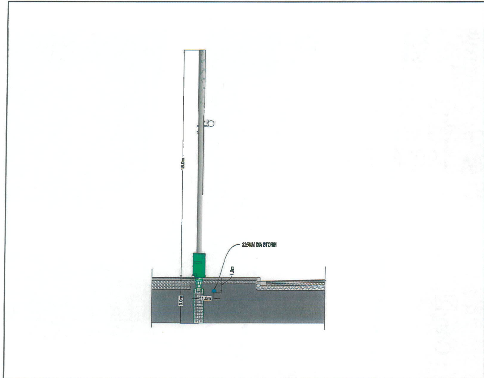
UNDERGROUND SERVICES SCALE 1:100
