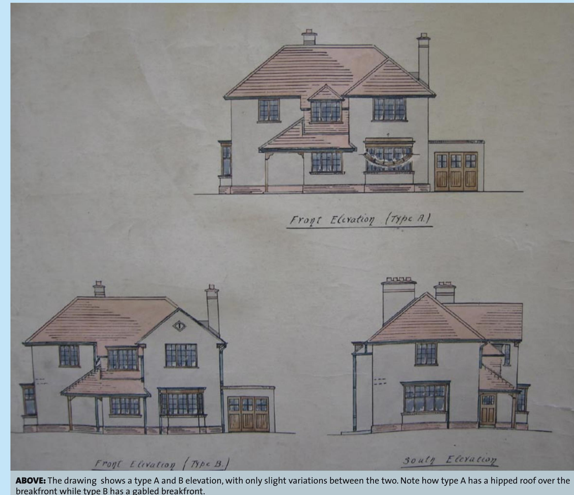
ABOVE: The drawing shows a type A and B elevation, with only slight variations between the two. Note how type A has a hipped roof over the breakfront while type B has a gabled breakfront.
