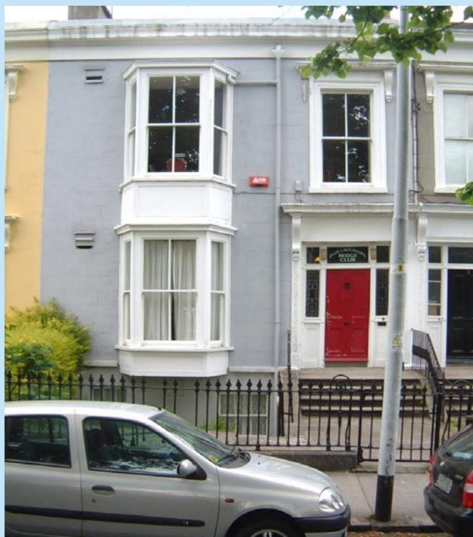
**ABOVE:** An example of the terraced two bay, two-storey over basement house on the north side, constructed with a shared chimneybreast party wall and having a paired front door with the neighbouring house.
