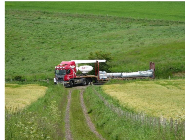
**Photograph 5: Wind turbine installation. Access roads to site will need to be assessed for suitability for long vehicles.**
