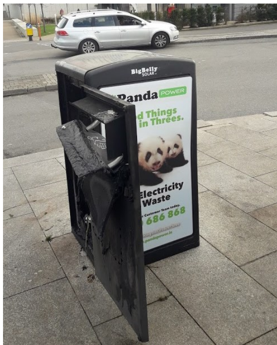
Fig. 2: Bin 50 on Queen's Road- after fire.
