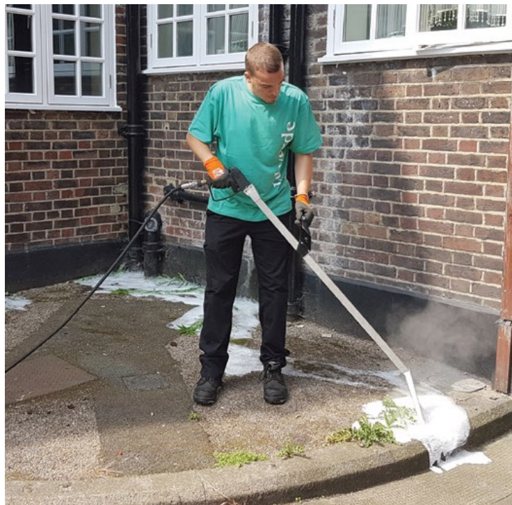
Fig 4: Hot Foam Application for Weed Control
