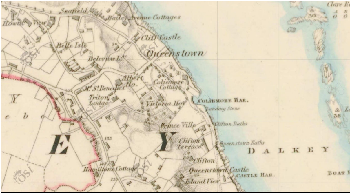
Figure 5: First edition Ordnance Survey surveyed in 1836 and published in 1843. Feint lines appear on historic map on same footprint of later masonry piers suggesting that at least planning (if not initial construction) for these structures to upgrade the harbour had commenced at this time.
