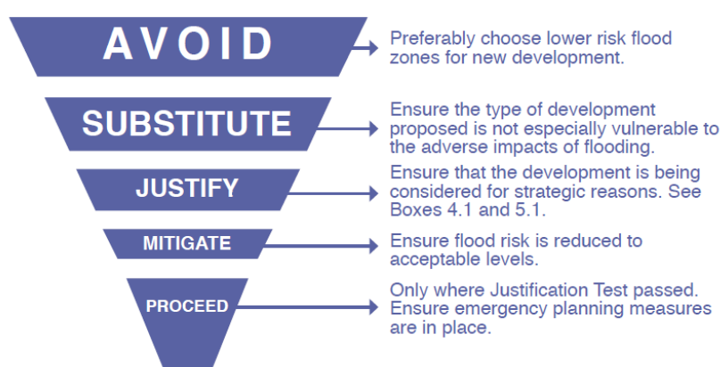
Figure 2-1: Sequential Approach Principles in Flood Risk Management
