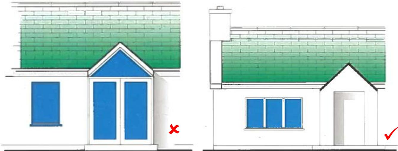
*The main entrance should be obvious. Where possible locate an entrance away from prevailing winds and/or on gable elevations. If using a porch, provide a simple, unobtrusive structure using the same materials as the dwelling and provide a pitched roof where appropriate.*
