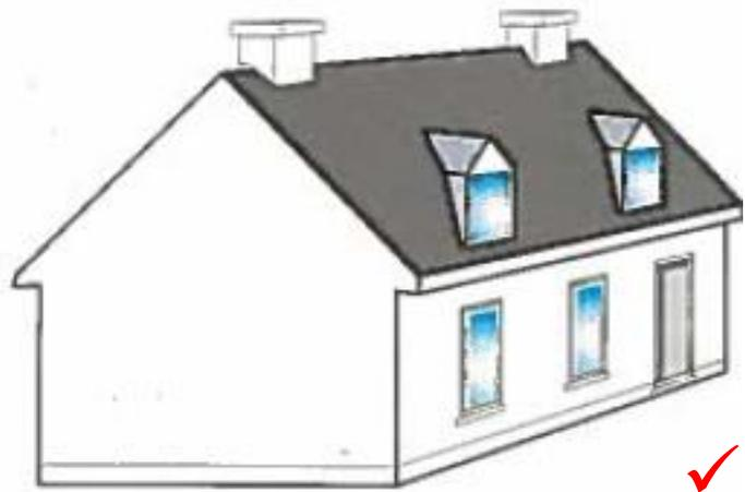
*Consideration should be given to using roof space for bedrooms where 2-storey dwellings are sought. This can reduce bulk and scale and provide dormers that successfully integrate into the roof from the outset.*
