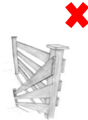
An example of an unsound stair guarding
