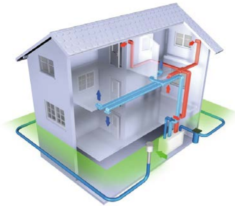
Figure 185. Ground-heat exchanger connected to ventilation system. Source: www.rehau.com .
