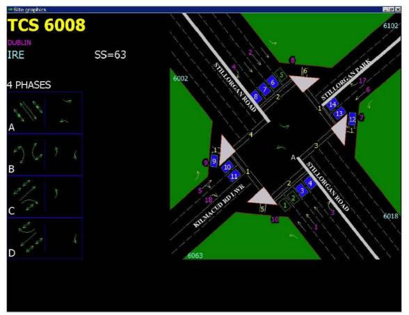
Figure 4.5 Existing Traffic Signal Plan
