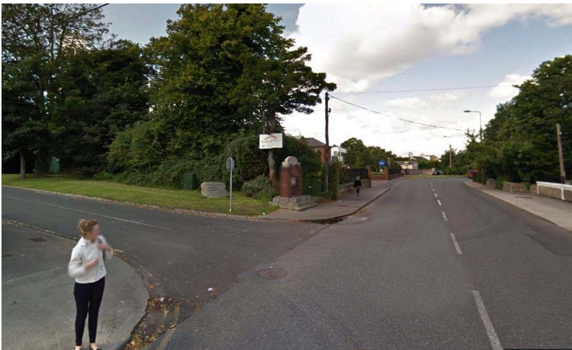
Figure 7.20: Limited footpath space, excessive road width
