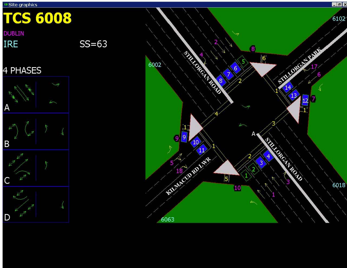
Figure 4.5 Existing Traffic Signal Plan
